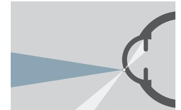
The angle between the illumination and the viewing axis should be as large as possible, and the slit to a minimum, for example 0.1mm or 0.2mm
