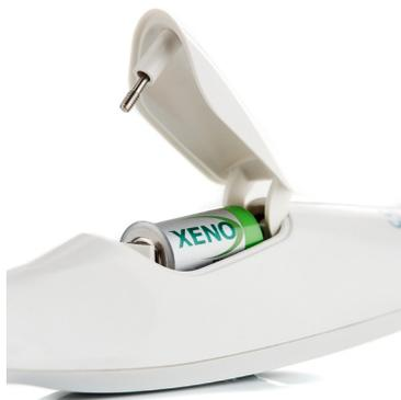
Figure 3.2 - Battery insertion
