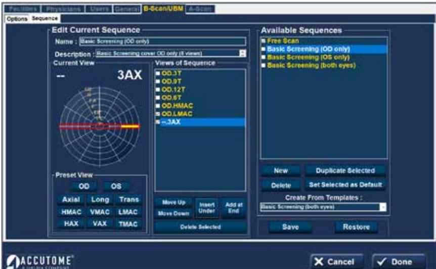
Figure 7.5 - Setup: B-Scan/UBM – Sequence – Change Probe Orientation
