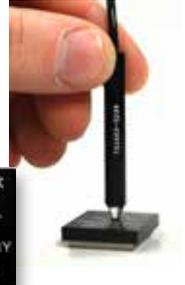
Figure 11.2 - Using the Pachymetry Test Block
