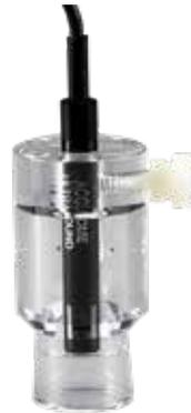
Figure 9.2 - A-Scan Probe with Immersion Shell
